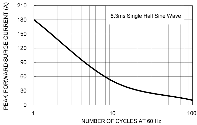
FIG. 7- MAXIMUM NON-REPETITIVE PEAK FORWARD SURGE CURRENT
